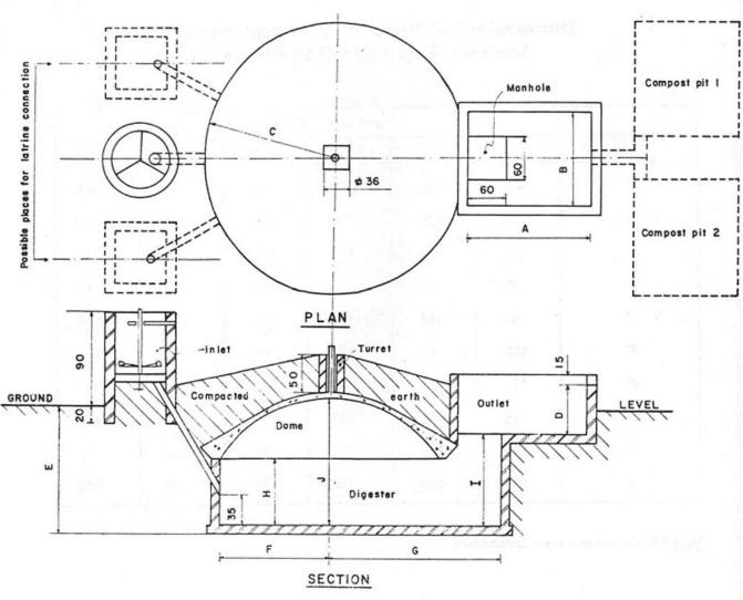
Figure 6.1: GGC 2047 model biogas plant
