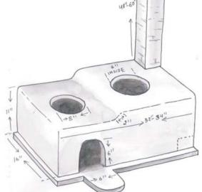
Figure 3.6 Two potholes ICS with grate Source : AEPC
