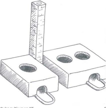
Figure 3.11: Three potholes multipurpose ICS
