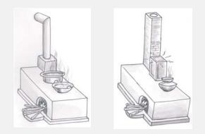
Figure 3.8: Metal chimney and use of tin for space heating
